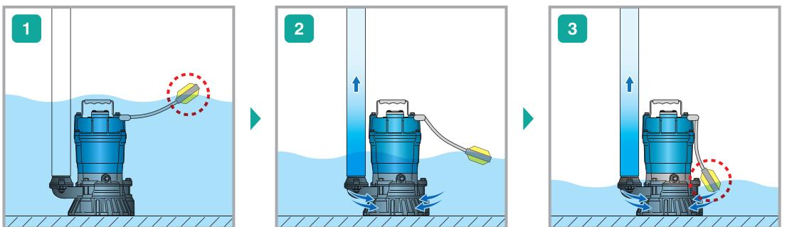
Pump starts operating when the water level rises to a preset level.
