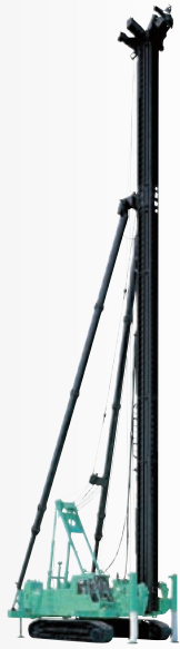
Pile Driving Rig
