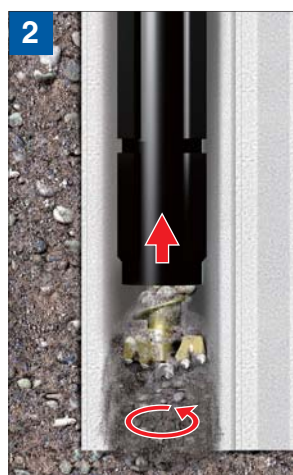
Extracting the Pile Auger after completion of sheet pile installation
